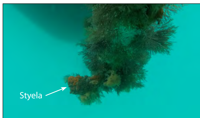
The bottom of the keel, especially in the case of yachts, can be heavily fouled even when the main hull is clean and well anti-fouled.
