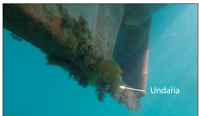
The bottom of the keel, especially in the case of yachts, can be heavily fouled even when the main hull is clean and well anti-fouled.
