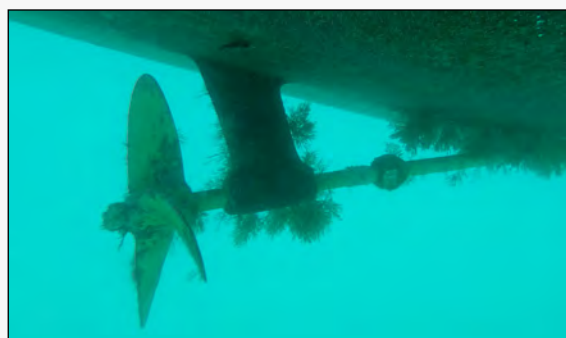
Some boats have a hull that appears clean, but can be fouled in 'niche' areas below the water-line.
