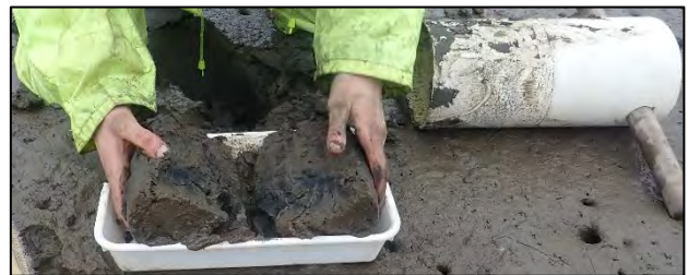
Measuring aRPD of a sediment core
