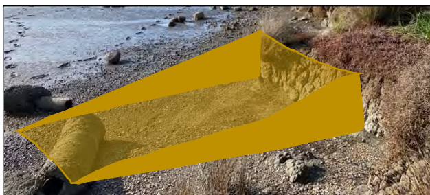
Illustrative cut and fill of the upper margin to increase planting habitat and reduce slope
