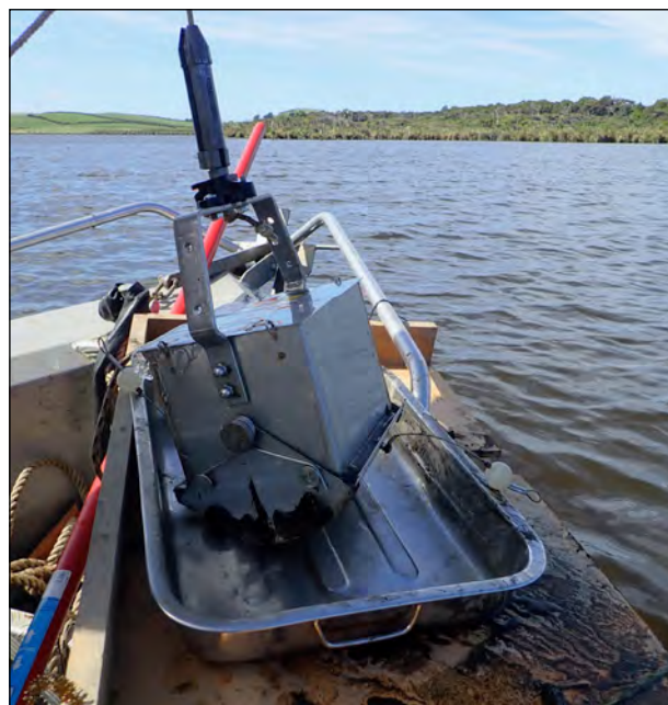
Ekman grab for sampling sediment in deep water
