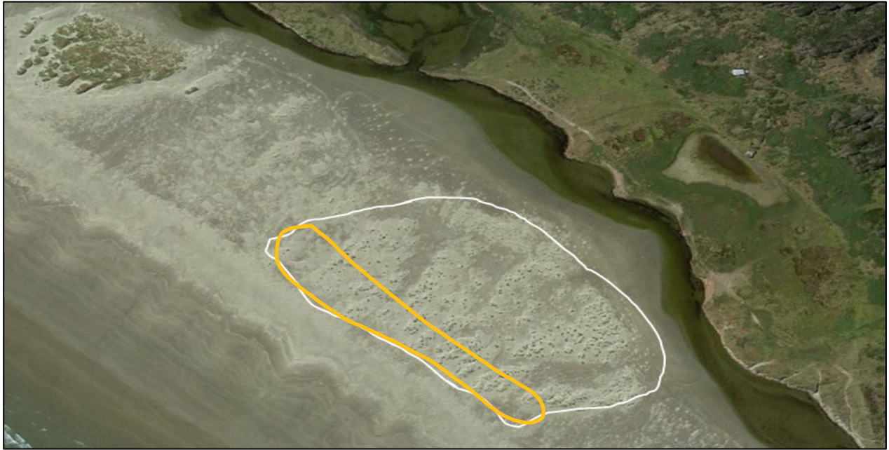
Fig. 12. The area of proposed dune restoration. Area of proposed initial planting highlighted in yellow (~5000m 2 ). Succession planting can occur after the establishment of the foredune plantings.
