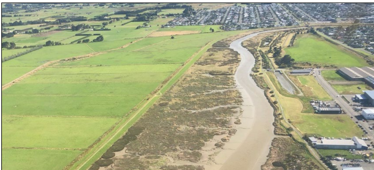
Upper Waihopai Arm showing remnant salt marsh within flood banks. The areas of green pasture either side of the channel is reclaimed estuary.
